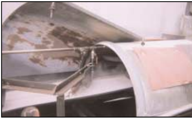
Chain mixing SoKleen® through batch of sand.
