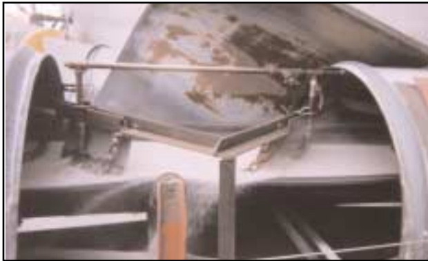
Blades and chain filtering SoKleen® through sand.
